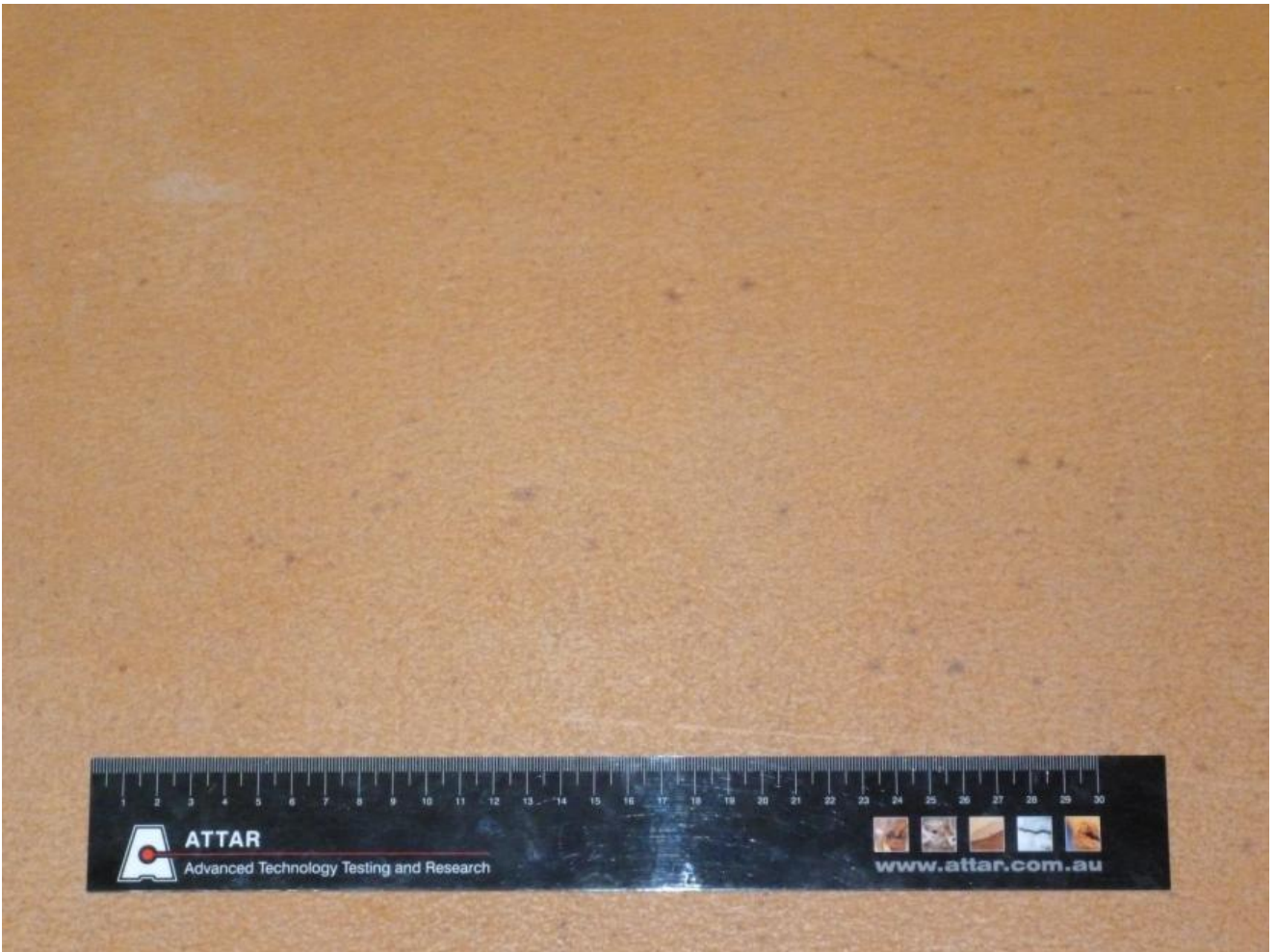
Figure 1: Intergrain UltraDeck Timber Stain – 2 coats with 5% Intergrain UltraGrip added to each coat applied to MDF board.
