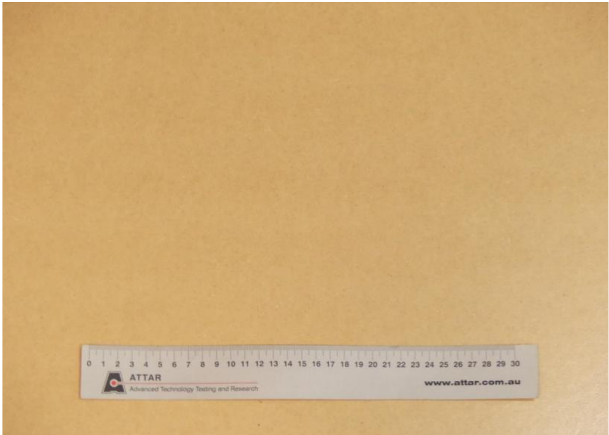
Figure 1: 2 Coats of Intergrain Slip Resistant UltraFloor applied to MDF board
