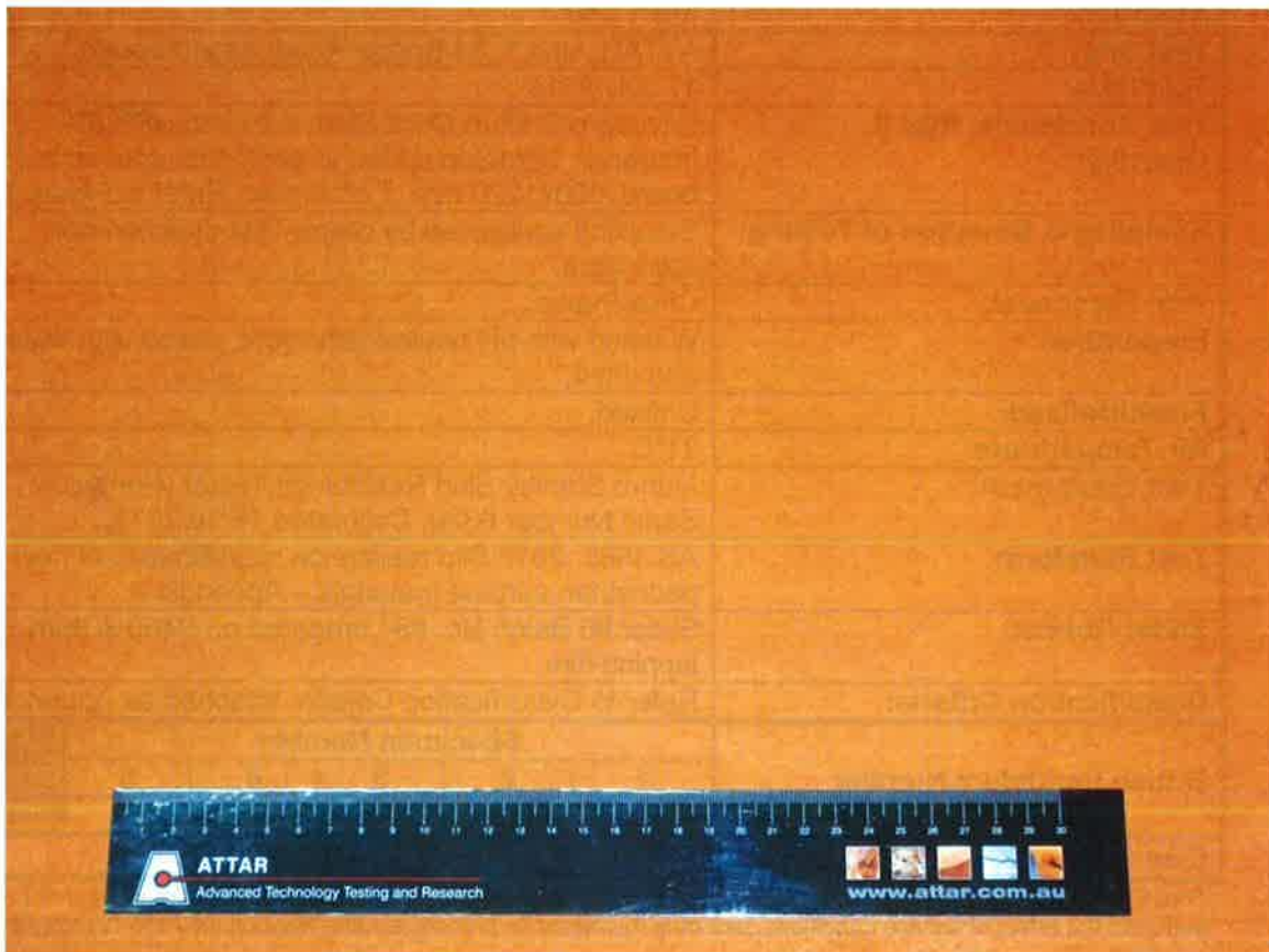
Figure 1: Enviropro Endure Deck Stain – 2 coats with 5% Intergrain UltraGrip added to each coat applied to MDF board.
