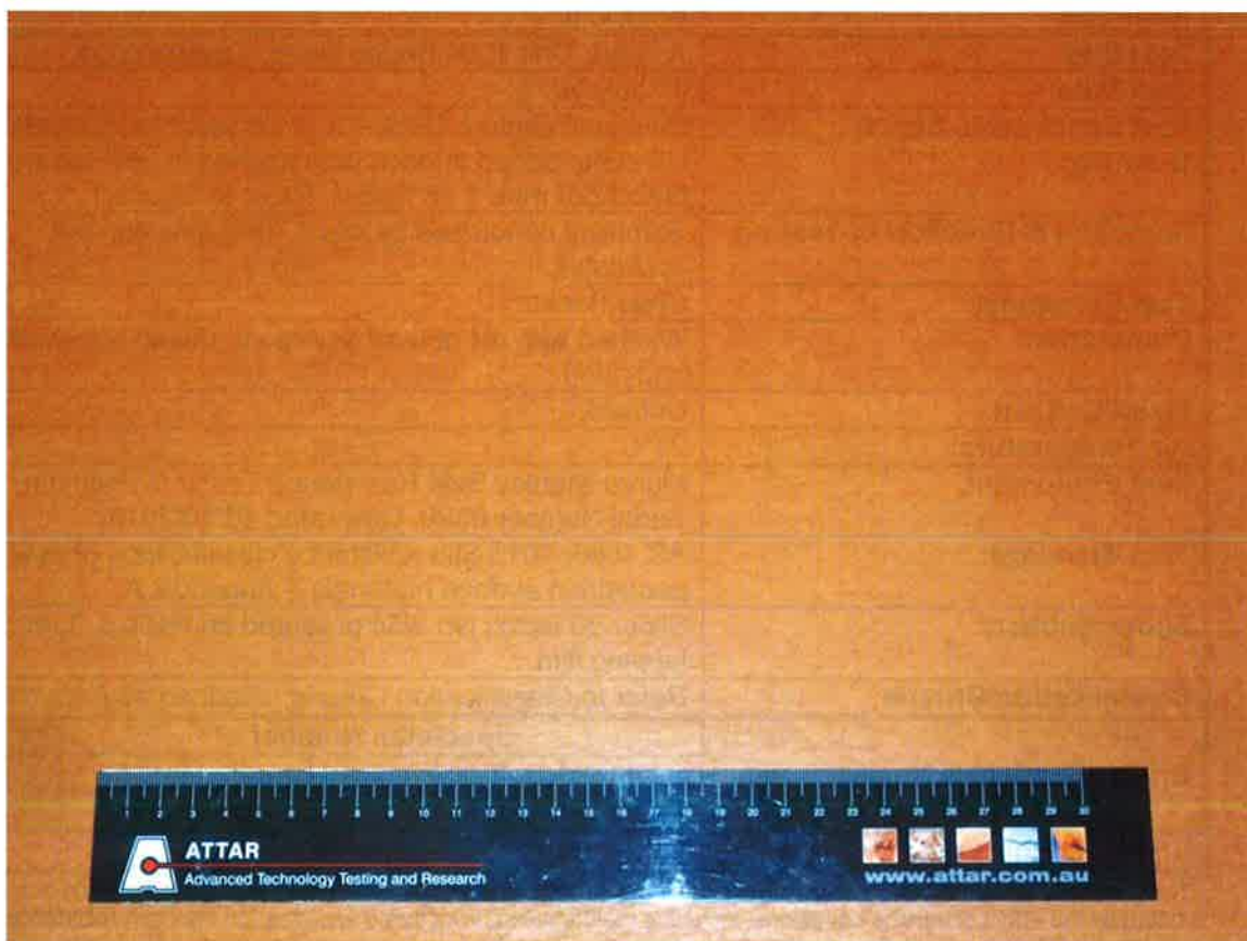
Figure 1: Enviropro Endure Deck – 2 coats with 5% Intergrain UltraGrip added to each coat applied to MDF board.
